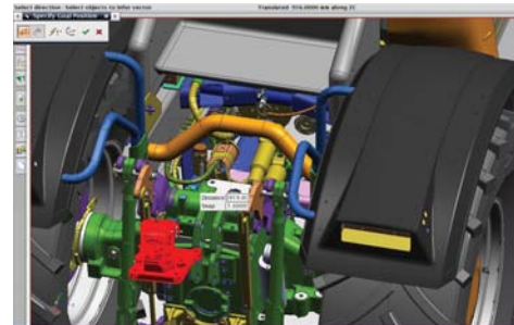
NX assembly validation tools include extraction path planning capabilities that optimize designs so that a product can be easily assembled, disassembled and maintained.
